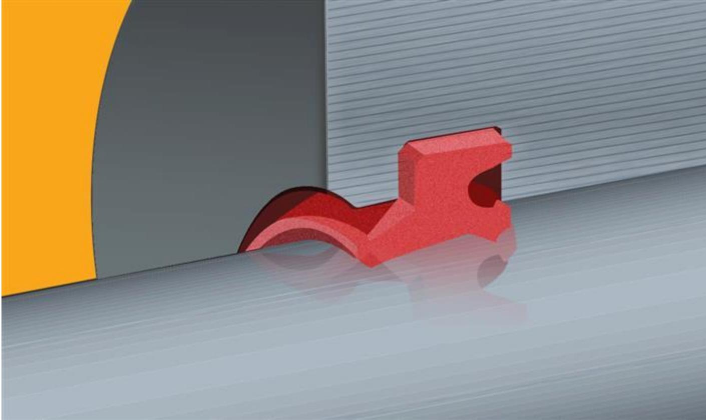
Hydraulic wiper seals are the first line of defense in many hydraulic systems. Unfortunately, they are also a perpetual problem for most users of hydraulic machinery. Microscopic scratches and gouges on the surface of cylinder rods can significantly reduce the life of wiper seals and give contaminants an easy path into the system. Particles as small as 5 microns can act like sandpaper on these surfaces, causing a chain of wear that grows exponentially in these fine-tolerance systems.
